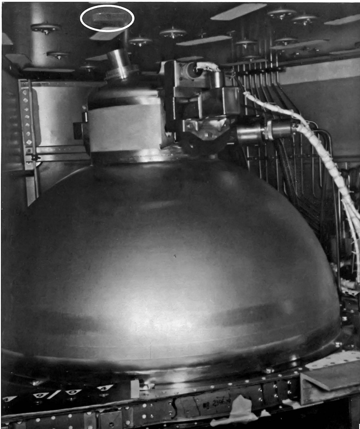
Figure C4-54.- Replacement oxygen shelf installed in Service Module 106. Note repairs to fuel cell shelf over oxygen tank no. 2.
