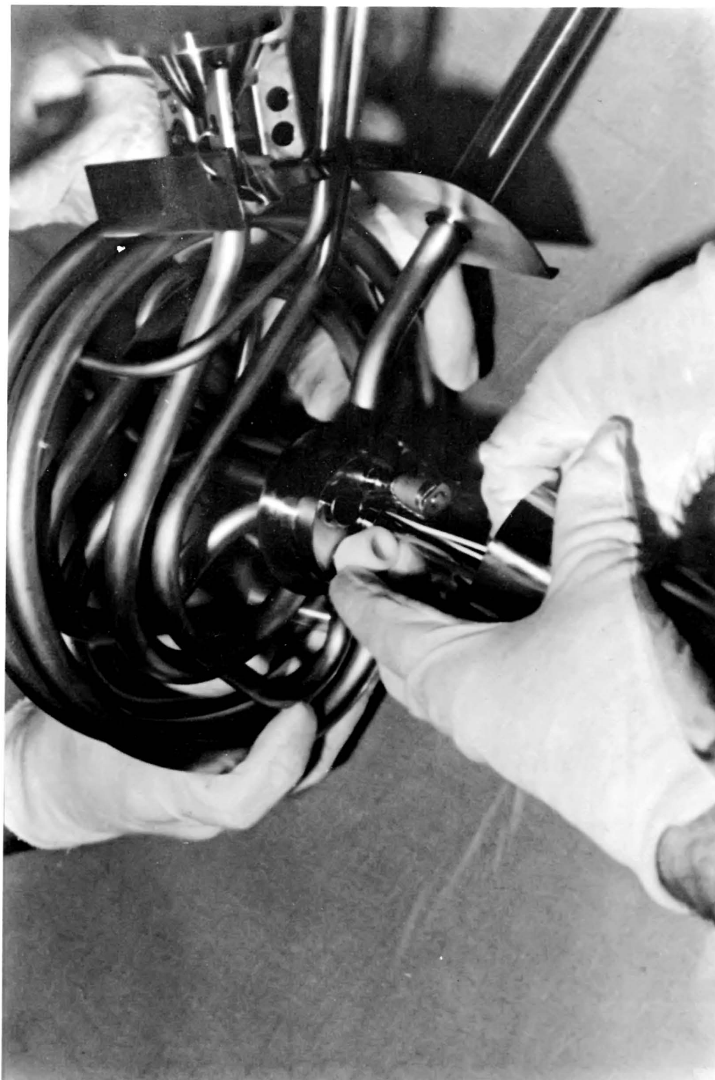
Figure C4-22.- Holding fill tube connecting parts in place.
