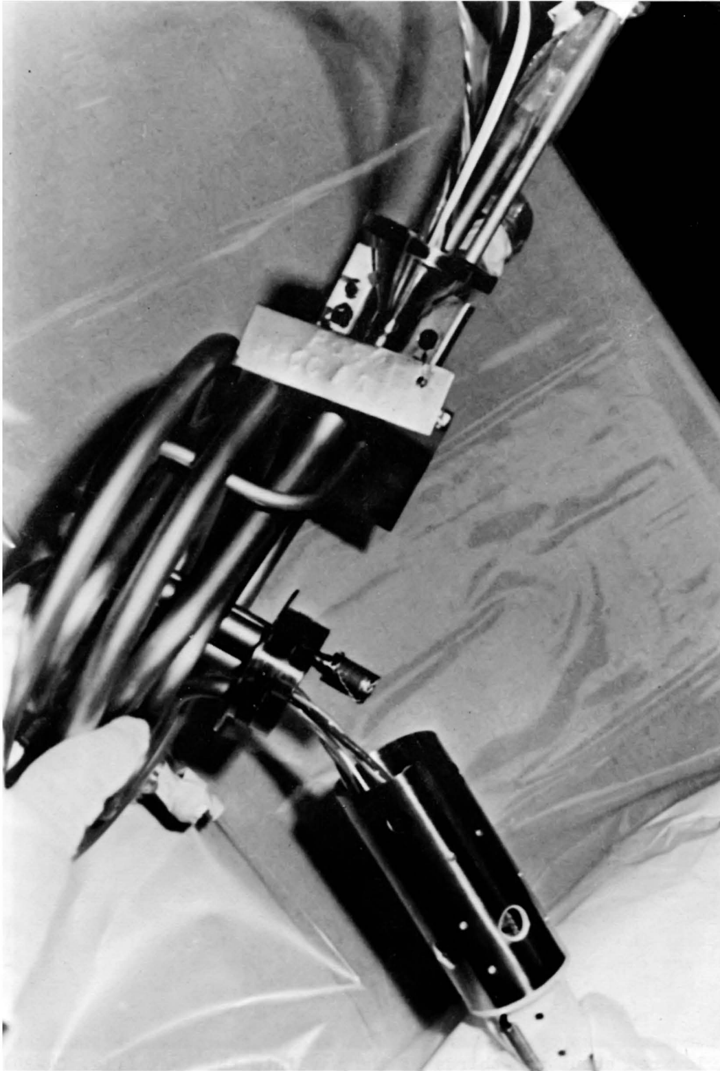
Figure C4-19.- Quantity probe and coil assembly ready to install fill tube connecting parts.
