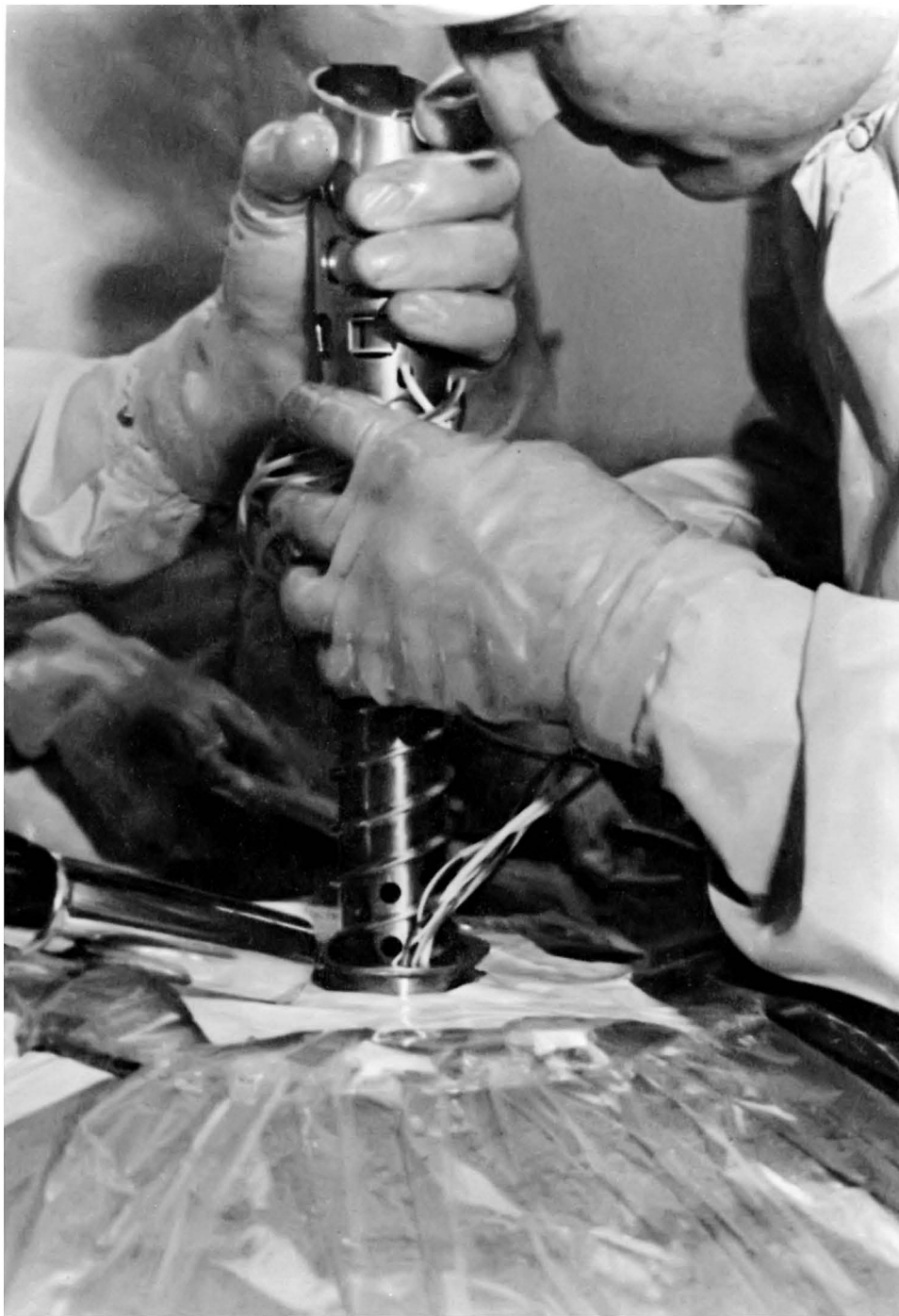
Figure C4-32.- Feeding wires into tank beside heater probe.
