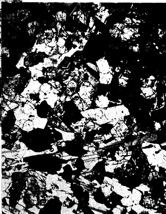
Figure 2. Photomicrographs of 15538,4 showing plagioclase-rich zone (bottom) and mafic-rich zone (upper). Widths about 3 mm. a) transmitted light; b) crossed polarizers.
