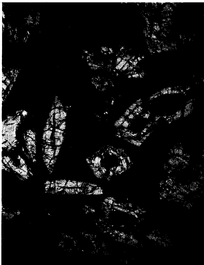
Figure 2. Photomicrograph of 15667,6. Width about 3 mm. Transmitted light. Most pyroxenes in thin sections seem to have been cut perpendicular to their long axes (indicating a lineation?) and no laths are seen.
