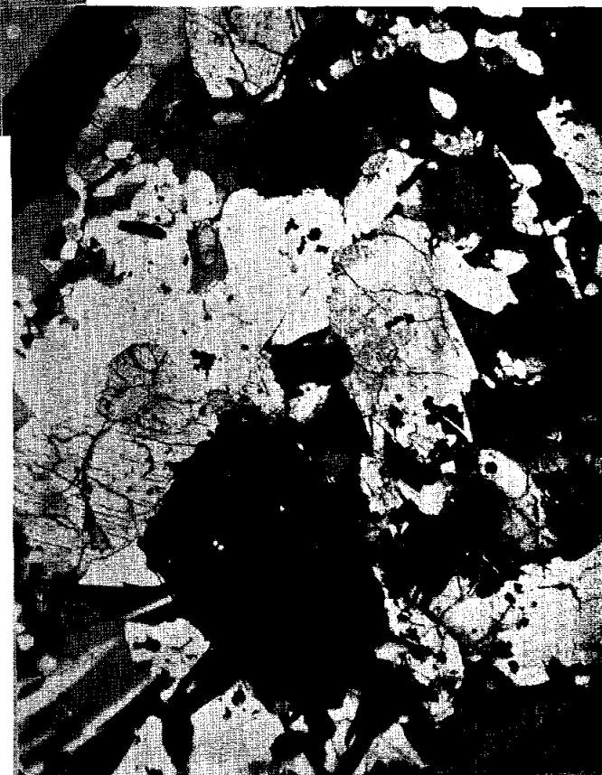
Figure 2. Photomicrographs of 15547,7. Widths about 5 mm. To left and upper right are euhedral olivines and some pyroxenes enclosed in plagioclase. Lower center is an anhedral, larger (about 0.5 mm) olivine. a) transmitted light; b) crossed polarizers.
