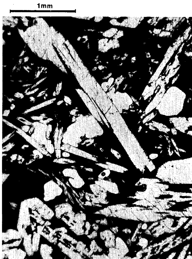
Figure 2. Photomicrograph of 15486,22, transmitted light, showing prismatic pyroxene phenocrysts, opaque groundmass, and vesicles.
